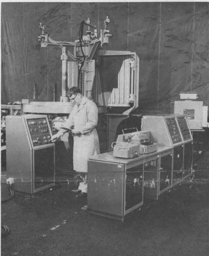
UNIVERSAL CONTOUR MEASURING MACHINE will be one of the major pieces of equipment to be installed in a new environmentally-controlled gaging and inspection enclosure at Livermore Laboratory. Photo shows the machine at manufacturer's plant.
